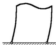
(c) Antisymmetrical (sway) mode of buckling
